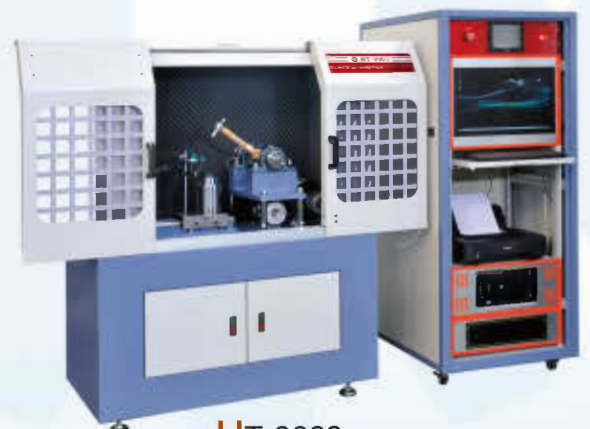
HT-3003 電腦伺服鐵錘敲擊 耐久試驗機 Computer Servo Hammer Striking Durability Tester
